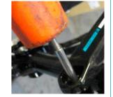
**B MOUNTING REAR TRIANGLE** Install the main pivot pin (female) from the drive side of the bike. Use a dead blow hammer to push the pin into place.
