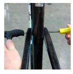
**2 REAR TRIANGLE DISASSEMBLY** Insert the guide pin tool into the 46.5 female bolt and use a dead blow hammer to tap the bolt out of the frame. Be prepared to catch the bolt as it exits the drive side of the frame. Leave the guide pin in the frame during the next step.
