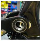
**T** MOUNTING REAR TRIANGLE Use the fox guide pin to align and hold the seatstays, dogbone, and shock together. Use a dead blow hammer to push the pin through the above mentioned components.
