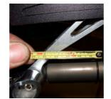
BOTTOM-OUT RESISTANCE The bottom-out adjuster has three full turns of adjustment. This adjustment controls the bottom out resistance of the shock, or the compression on the final part of the shock's stroke. If you feel like you are bottoming-out the shock on big hits, you can minimize this sensation by increasing the bottom-out resistance.
