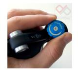
**REBOUND** The rebound adjustment has a nine click range. As a general rule, adjustments that are too fast (counter-clockwise) will produce a springy ride with excessive kick-up of the rear end. Adjustments that are too slow (clockwise) will cause packing of the rear wheel and give the bike a sluggish feel.
