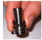
LINKAGE ASSEMBLY Place the dogbone over the shock with the counter-bored holes facing out, what would be back towards the seat tube, and the threaded end facing towards the shock. Slide the pin subassembly into the shock eyelet as shown.
