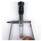
FRAME DISASSEMBLY Slide a washer and removal slug onto the threaded bolt. Slide this subassembly through the shock and dogbone. On the opposite end, slide on the catch sleeve, washer and then thread the nut on.
