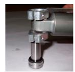
LINKAGE ASSEMBLY Once you have the pin subassembly started into the shock eyelet, you can slide the threaded bolt, press-cup and press-cup insert configuration from step one through the steel pin subassembly and shock. On the opposite end of the bolt, slide a second nylon washer, the remaining two bearings, press-cup insert, press-cup, washer and nut.
