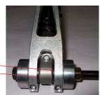
TINKAGE ASSEMBLY Use two 1/2" wrenches and torque the linkage together until the bearings press into position. Make sure bearings are flush on both sides of dogbone. This will ensure proper alignment of the swing arm once it is installed.
