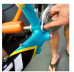
FRAME ASSEMBLY Install the black washer and button head bolt over the main pivot pin as shown. Cinch the button head down with a 5mm allen key while holding the main pivot with 6mm allen key.
