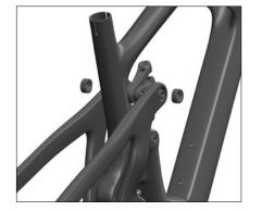
Install Large Collet Wedge Bolts (3.9) into 2x Collet Axles (3.1) and (3.4).
