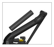
Install Battery (4.6.2) into the downtube. Battery should clip in firmly and latch without pinching any wires or housing. Install Battery Guard (4.7) onto the Battery using 4x M4 BHCS (4.63). Snug the 4x BHCS until hand-tight.
