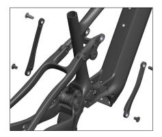
Install Timing Link (4.4) and Timing Link (4.5) onto the Rocker Link Assembly using 2X Tie Link Bolt, Long (4.61) and to the Switch Link Assembly (4.1) using 2X Tie Link Bolt, Short (4.10).
