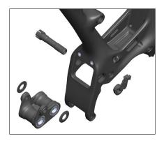
Lightly grease the bore and collet nut interface on the Front Triangle main pivot interface Install Lower Switch Link Assembly (4.1) with two Race Extenders (4.15) into the Front Triangle and secure with 15mm Collet Axle (4.8) and Chain guide Mount Collet Nut (4.47).
