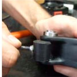
**2 DOG & SHOCK MOUNTING ASSEMBLY** Now insert 23.5mm reducers into shock and hammer into place with dead blow hammer. Twist lower portion of shock 180 degrees so white screw is pointing downward in relation to valve core.
