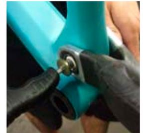
**4 SHOCK & DOGBONE DISASSEMBLY** Remove the guide pin from shock, dogbone and seatstay junction. Once you remove the guide pin, be prepared to catch swing arm. TO remove the shock and dogbone mountain bolts, place two 5mm allen keys on both ends of the bolt and turn counter clockwise. Once the male Yeti bolt is removed, take a 6mm allen key or Fox toll and tap out the female end.
