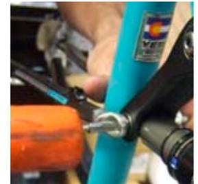
**8 MOUNTING REAR TRIANGLE** Install the main pivot at this point from the drive side of the bike. Use your dead blow hammer to hammer into place.
