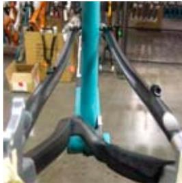
**Tip:** If there is any binding during the installation of the Ti stud, loosen the dogbone and seatstay pinch bolts to relieve the binding pressure during the installation process. If loosened, make sure the alignment is correct before tightening pinch bolts down.
