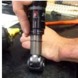
**4 DOG & SHOCK MOUNTING ASSEMBLY** Hang shock and dogbone assembly off of frame. Insert 34.0mm Ti female bolt through drive side (The right side when standing behind the seat tube) for the shock. Use Ti male bolt on non-drive side to tighten shock into place with 5mm allen key while supporting lower end of assembly.
