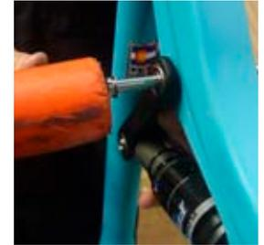
**6 REAR TRIANGLE ASSEMBLY** Press the bearings into the seatstays of the rear triangle with shoulders facing in. Slide the swing arm over the main pivot using the indentations in the swing arm to align.
