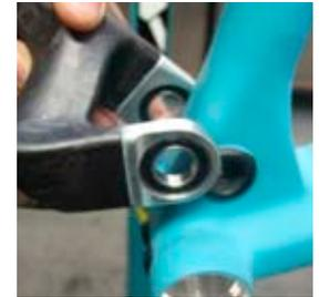
**7 MOUNTING REAR TRIANGLE** Install the Fox Guide Pin in the seatstays, dogbone and shock to hold and align the three together. Use a dead blow hammer to hammer into place.
