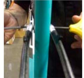
**2 REAR TRIANGLE DISASSEMBLY** Insert Fox Guide Pin into Ti stud and use dead blow hammer to knock out of place. Be ready to catch the Ti stud as it exits the drive side of the bike.
