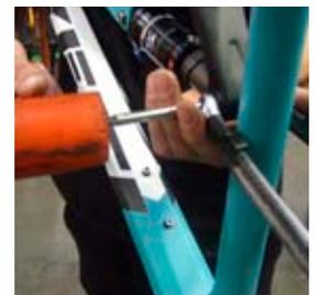
**3 SHOCK & DOGBONE DISASSEMBLY** Back the main bolt all the way off of the main pivot bolt. Use punch and dead blow hammer to remove the main pivot. Hammer the male bolt so the main pivot exits the drive side of the bike.
