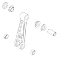
**DOGBONE ASSEMBLY** Press the dogbone bushing insert (8) into the Igus bushings (22) until there is equal amount of insert sticking out each side of the Igus bushings [22].
