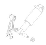
Figure 3a: Dogbone (2) and Shock (3) Assembly with Fox Pin (10) and Black Nvlon Washers (11), exploded
