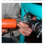
Double-check pinch bolts on the dogbone and tighten down with 2.5mm allen key. Double-check tightness of all other bolts.
