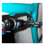
FRAME DISASSEMBLY Hammer in Fox guide pin with dead blow hammer. Be prepared to catch female bolt as it exits the non-drive side of the hike
