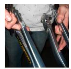
FRAME DISASSEMBLY Loosen up the male bolt from the main pivot.
