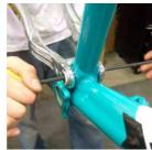
Make sure bearings on rear chainstay is flushed with metal of chainstay. Install seatstay with "Yeti" logo facing out above the dropout.
