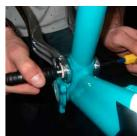
**FRAME DISASSEMBLY** Slide chainstay off of rear indentions. Separate dogbone and shock.
