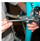
FINISHING TOUCHES Use dead blow hammer to hammer female stud through. Be ready to catch as it exits the non-drive side of the bike.
