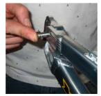
Screw male bolt into Ti female stud. Slide a 8.5mm ID washer Ti female stud
