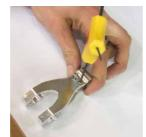
**REAR TRIANGLE ASSEMBLY** Tighten down with Ti male bolt and 2.5mm allen key.
