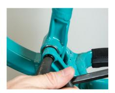
**08.** Tighten the pivot axle using a 10mm hex wrench.
