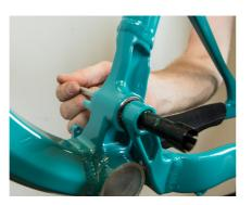
**06.** Partially install the Pivot axle from the non-drive side. Use a Guide Pin tool to help align the bearing spacer sleeve from the drive side.
