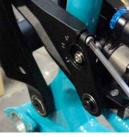
16 CHAINSTAY PROTECTOR The 303 RDH has a bolt-on chainstay protector. Install the chainstay protector on the driveside chain stay using two 4x.7x8 bolts.
