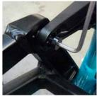
**MAIN ASSEMBLY** Tighten four male 12.7mm x 12 mm pivot pin caps into the female pivots pins on the push links and car mount. Prep the male threads with grease. Torque: 65-70in/lbs. At this point the rear triangle will be able to move freely on the rail system. Ensure the car does not dent the seat tube.
