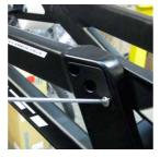
**MAIN ASSEMBLY** Slide the front of the shock into the frame mount. Attach the shock to the frame with a M6 x 31mm Ti female bolt and a M6x1x12 Ti male bolt. Use the guide pin tool to align the shock in the frame while inserting the female bolt.
