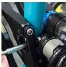
MAIN ASSEMBLY Using a dead 14 blow hammer push the 57.5 bolt through the eccentrics and shock. Use two 5mm allen keys to tighten the shock with a M6x1x12 Ti male bolt prepped with locktite.
