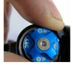
**HIGH SPEED COMPRESSION** The HSC adjuster has a twelve click range that can be adjusted by inserting a 2.5mm allen key into one of the angled holes. The HSC adjuster mainly affects the compression damping during medium-to-fast suspension movements.
