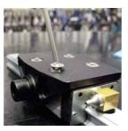
**2** MAIN ASSEMBLY Attach the rail sub assembly to the frame with three 4x.7x16mm socket head bolts. Prep the bolt threads with locktite. Tighten the bolts using a 3mm allen key. Torque: 40in/lbs
