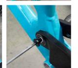
**MAIN ASSEMBLY** Press a 12.7mm x 18mm pivot pin through each of the bearings located at the top of the seat stays on the rear triangle. Orient the pin so the exposed female threads are on the inside of the seatstays.
