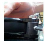
DOG & SHOCK MOUNTING ASSEMBLY Use a dead blow hammer to install two 23.5mm reducers into the lower portion of the shock.
