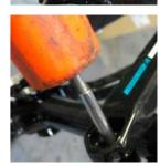
**MOUNTING REAR TRIANGLE** Install the main pivot pin (female) from the drive side of the bike. Use a dead blow hammer to push the pin into place.
