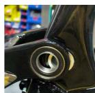
**MOUNTING REAR TRIANGLE** Use the fox guide pin to align and hold the seatstays, dogbone, and shock together. Use a dead blow hammer to push the pin through the above mentioned components.
