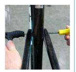
REAR TRIANGLE DISASSEMBLY Insert the guide pin tool into the 46.5 female bolt and use a dead blow hammer to tap the bolt out of the frame. Be prepared to catch the bolt as it exits the drive side of the frame. Leave the guide pin in the frame during the next step.
