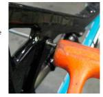
REAR TRIANGLE ASSEMBLY Slide the swingarm over the main pivot bore, using the grooves in the swingarm to properly align over the bore
