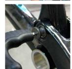
SHOCK & DOGBONE DISASSEMBLY Remove the guide pin from the seatstay junction and then pull the rear triangle off of the frame. Remove the male bolt from the 40.5mm Ti female bolt holding the dogbone in place. Use the guide pin and a dead blow hammer to tap the female bolt out of the frame. Repeat the process for the bolts holding the shock in place.
