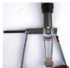
FRAME DISASSEMBLY To remove the main pivot pin, place a 5mm allen key on the button head bolt and a 6mm allen key on the pivot pin. Turn counter-clockwise until the button head is removed. Then take an 8mm allen key and tap out the main pivot pin.
