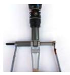
**2 LINKAGE DISASSEMBLY** Place the wrenches on the tool assembly and turn to press the pin out.
