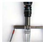
LINKAGE ASSEMBLY When turning the tool make sure you press the shock pin into the correct position. The easiest way to gauge this is to use one of the nylon washers. The relief on the pin should be even with the washer.
