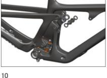
Place 2x Race Extenders (3.5) onto the upper bearings in Link Assembly (3.16). Rotate Rear Triangle and Link together, lining up SS Pivot bores.
