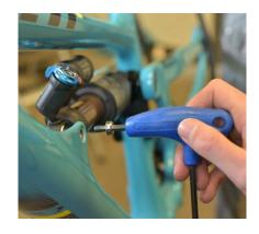
17. Secure front shock mount with Titanium Male Bolt (300030151) prepped with Blue 243 Loctite and Washer (300030062).
