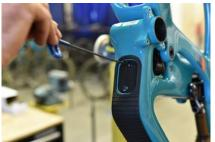
**01.** With a 3mm allen key, remove the lower cable port access cover near the bottom bracket.
