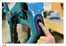
Use your finger to help push the housing around the bend in the frame up into the seat tube.
