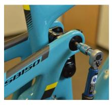
**12 c.**Torque Seatstay Pivot Female Bolt to *16 Nm*Repeat process for opposite side.
