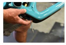
Drop a Park Tool Router tool down the seat tube until it exits the access port.
