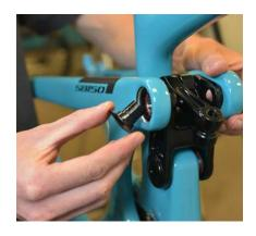
**12a.**Grease shaft of 2x Seatstay Pivot Female Bolt (200020326).
