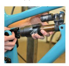
**13.**Open the Upper and Lower Shock Extenders and position the Shock into the frame, allowing it to sit between the two Extender jaws. Secure front eyelet with a Guide Pin
