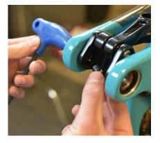
**12 b.**Rotate Swingarm Forward and move Upper and Lower Shock Extenders out of the way.
