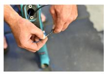
Outside of the access port, connect the Park router tool to the housing.
