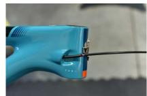
At the same time, pull the shifter housing out of the head tube port while pushing the seatpost housing into the seat tube until the double barb exits the head tube.
