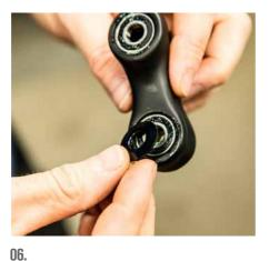
Place the bearing race extender washers (300020049) on the lower link bearings. There should be just enough grease there to hold the washers in place.
