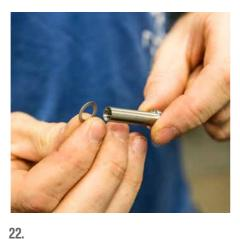
Place the 8.5mm washer (300030069) on the front shock mounting pin (300030262) and lightly grease the pin shaft.
