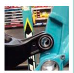
MOUNTING REAR TRIANGLE Install the main pivot pin from the drive side using a dead blow hammer. Be sure to lightly coat the pivot pin with grease. Thread the main pivot pin cap into the non drive side of the pivot pin. Use a generous amount of grease on the male threads. Tighten the pin and cap with two 5mm allen keys. Torque 115-125 in/lbs
