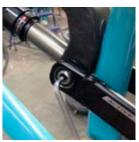
REAR TRIANGLE DISASSEMBLY Insert the guide pin tool into the stainless female bolt and use a dead blow hammer to tap the bolt out of the frame. Be prepared to catch the bolt as it exits the drive side of the frame. Leave the guide pin in the frame during the next step.
