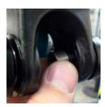
SHOCK MOUNTING ASSEMBLY Rotate the bottom of the shock into the dogbone and seatstay. Use the guide pin tool to align the shock, dogbone, and seatstay. Insert the female M5x44 stainless shock bolt through the drive side of the frame. Apply locktite to the male M5x12 stainless shock bolt and tighten the assembly with two 5mm allen keys.
