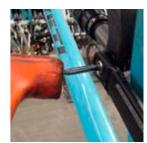
**REAR TRIANGLE DISSASSEMBLY** Remove the male main pivot bolt from the female main pivot pin with a 5mm allen key. Use a punch and a dead blow hammer to remove the main pivot pin from the chainstay and front triangle.
