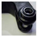
DOGBONE & SHOCK MOUNTING ASSEMBLY Insert two 22mm reducers into the shock and tap into place with a dead blow hammer.
