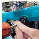
SHOCK AND DOGBONE DISSASSEMBLY Remove the Ti male bolt from the 31.0 female Ti bolt holding the shock on the frame using two 5mm allen keys. Insert the guide pin tool into the female bolt and use a dead blow hammer to tap the bolt out of the frame. Be prepared to catch the bolt as it exits the drive side of the frame
