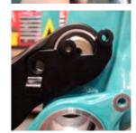
ASR7 FRONT DERAILLEUR MOUNT Attach the mount with a Ti female M6x16.5 bolt and a M6x1x12 Ti male bolt. Ensure each bolt has the proper washer installed. Prep the male bolt with locktite and tighten the assembly with two 5mm allen keys.
