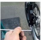
ASR7 FRONT DERAILLEUR MOUNT Insert the front derailleur mount into the drive side chainstay yoke. Ensure the cable guide on the mount is facing out.
