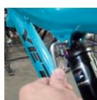
**AXLE SYSTEM** Slide the threaded axle through the non drive side of the frame and the hub. Lightly grease the threads on the axle and tighten into the axle nut on the drive side of the frame with a 5mm allen key. Torque 40-45 in/lbs
