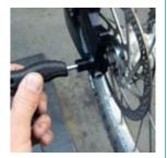
**AXLE SYSTEM** Tighten the pinch bolt on the non drive side dropout to secure the axle. Use a 5mm allen key. Torque 75-85 in/lbs
