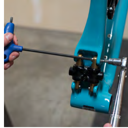
09. Use a ball-end wrench to prevent the inner Ti Female Bolts from rotating. Torque the 4x Flat Head Ti Male Bolts to 12.5 - 14 Nm .
