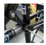
REAR TRIANGLE DISASSEMBLY Insert the guide pin tool into the 46.5 female bolt and use a dead blow hammer to tap the bolt out of the frame. Be prepared to catch the bolt as it exits the drive side of the frame. Leave the guide pin in the frame during the next step.
