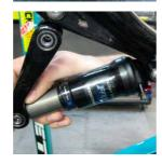
DOGBONE AND SHOCK MOUNTING ASSEMBLY Install the dogbone using a 40.5mm Ti female bolt and a Ti male bolt. Orient the dogbone so the flat surface of the part is facing the rear of the frame, and use a dead blow hammer to insert 40.5mm female bolt through the top of the dogbone and the frame. Use the Ti male bolt on the non-drive side to tighten the dogbone into place with a 5mm allen key. Torque: 90-95 in/LB
