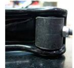
**2 DOG & SHOCK MOUNTING ASSEMBLY** Use a dead blow hammer to install two 23.5mm reducers into the lower portion of the shock.
