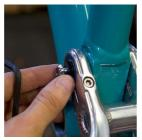
FRAME ASSEMBLY Tighten down the pin and button head with a 5mm and 6mm allen key. The 6mm allen key is used for the pivot pin and the 5mm allen key is used for the button head.
