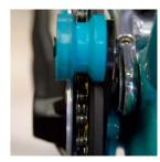
**7 FUNCTION CHECK** Now that the setup is complete spin the cranks to check the function of the chainguide. The rollers should move freely and the chainline should be straight when shifted to the middle cog on the cassette.
