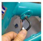
FRAME ASSEMBLY Place the head of the shock into position on the mounting tabs as shown.
