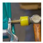
FRAME ASSEMBLY Place the Pivot Pin Washer over the exposed end of the pin on the non-drive side. Then thread the Button Head Bolt (M6 X 1 X 12 mm) into the pin.
