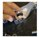
FRAME ASSEMBLY Slide the Dogbone and bearing assembly in the frame. Making sure ti line up the bearing thru-hole with the frame mount thru-hole.
