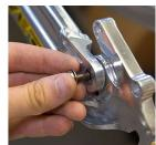
**FRAME ASSEMBLY** Secure the male and female bolts using two 5mm allen keys.
