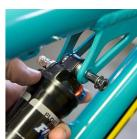
FRAME ASSEMBLY Thread the Pivot Bolt Male Yeti (M6 X 17 mm) and Washer (8.5 X 12.5 X 0.5 mm) in the female bolt and secure using a Two 5mm allen keys.
