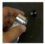
LINKAGE ASSEMBLY Once both bearings and in the proper position secure the bearings via the pinch bolts. Tighten the Bolt Cap M3 X 0.5 X 12 mm using a 3mm allen key.
