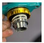
SPACER SETUP On non drive side install the threaded cup. On the crank arm with the attached spindle install two white spacers and one black spacer. Then lube the spindle and tap it into the threaded cups.
