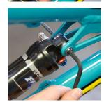
**FRAME ASSEMBLY** Secure the main pivot bearings via the pinch bolts. Tighten the Bolt Cap M5 X 0.8 X 24 mm using a 4mm allen key.
