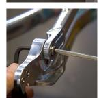
FRAME ASSEMBLY Before making the final connection thread one the remaining Bolt-Ti-Male (M6 X 1 X 12 mm) and Washer (8.5 X 12.5 X 0.5 mm) into the Stud-Ti-Female (M6 X 8 X 53 mm). Just secure finger tight. The purpose is to create a bolt sub-assembly for the final connection.
