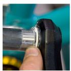
**GUIDE POSITION** Attach the boomerang to the ISCG mounts using the flat head socket cap screws. The boomerang should be rotated so the top arm of the boomerang is in line with the 4X seatube. You do not need any washers between the frame and the boomerang for spacing.
