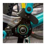
SPACER SETUP Once you have the spindle through both cups place one black spacer, two white spacers, and one red spacer on the spindle. Then attach the chainring and bashguard to the drive side crank arm. Lube the splines and install the drive side crank arm to the spindle.
