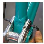
FRAME ASSEMBLY Place the seatstays onto the chainstay assembly. Line up the thru-holes on the seatstay with the inner race of the bearings on the chainstay.
