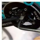
SPACING CHECK Once the drive side crank arm is securely fastened, check the spacing. The boomerang rollers should be centered over the chain and there should be the same pacing between the boomerang guides and chain as there between the bashguard and chain.
