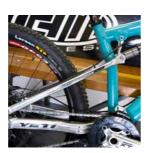
**REAR BRAKE** The rear brake loops across the head tube and into the first open cable stop on the down tube. The line is the run along the downtube in the second and third open cable stops.
