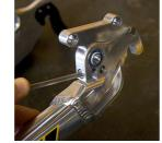
FRAME ASSEMBLY Slide the swingarm assembly into position on the frame as shown. Make sure to line up the inner race of the bearings with the thru-hole on the frame.
