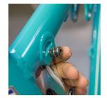
FRAME ASSEMBLY Thread the Pivot Bolt Male Yeti (M6 X 17 mm) and Washer (8.5 X 12.5 X 0.5 mm) in the female bolt and secure using a 5mm allen key
