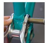
FRAME ASSEMBLY Tap the pin through the bearings and frame via a dead blow hammer.
