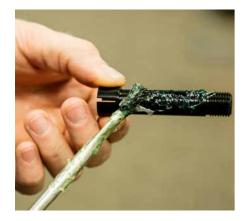
Grease the main pivot collet axle (300040485), including the threads.
