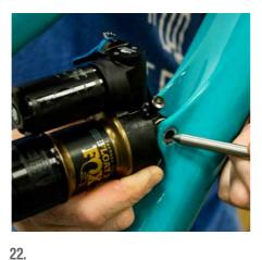
Align the front shock eyelet to the mounting points on the front triangle and secure with a guide pin.
