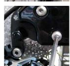
**DROPOUT ADJUSTMENT** Double check that the dropouts are square and the rear wheel is centered in the frame. Ensure that the dropout bolts are torqued to spec.
