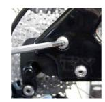
**DROPOUT ADJUSTMENT** Loosen the two M6x34mm tension bolts located above the back of the chainstay on each side of the bike.
