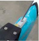
**MAIN ASSEMBLY** Slide the swingarm over the main pivot, using the grooves in the swingarm to properly align over the bore.
