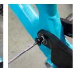
**5** MAIN ASSEMBLY Press a 12.7mm x 18mm pivot pin through each of the bearings located at the top of the seat stays on the rear triangle. Orient the pin so the exposed female threads are on the inside of the seatstays.
