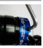
More Resistance – clockwise rotation Less Resistance – counter-clockwise rotation
