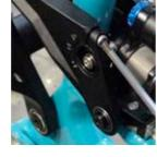
**ECCENTRIC ADJUSTMENT** Place a 5mm allen key into each eccentric insert as shown. Rotate the eccentric to the desired position. The eccentric adjustment has a range of 64° / 13.85″– 65° / 14.35″.
