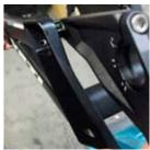
**MAIN ASSEMBLY** Rotate each of the push links towards the front of the frame and align the bearing in the link with the pivot pin on the car mount. Flex the link over the pivot pin on the car and tap into place with a dead blow hammer.
