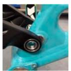
MAIN ASSEMBLY Install the main pivot pin from the drive side using a dead blow hammer. Be sure to lightly coat the pivot pin with grease. Thread the main pivot pin cap into the non drive side of the pivot pin. Use a generous amount of grease on the male threads. Tighten the pin and cap with two 5mm allen keys. Torque 100 in/lbs
