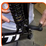
Take the dickey tool (or an 8mm allen key) and line all three components up by inserting the tool through the discs. Place the shock into position and tap the female Yeti bolt through the discs and the shock eyelet. Thread the button head bolt (6x1x12) into the female Yeti bolt and cinch the assembly down with two 5mm allen keys.
