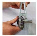
LINKAGE ASSEMBLY Slide a washer of the linkage tool (200020071) on the threaded bolt then slide this through the removal slug (1.5" long). Then slide on the shock pin. Slide the tool assembly through the dogbone and shock eyelet. On the opposite side slide on the catch sleeve and washer, and then the nut. Place the wrenches on the tool assembly and tighten, installing the shock pin.
