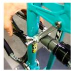
FRAME ASSEMBLY Make sure the bearings are lined up with the main pivot before tapping the lightly greased main pivot pin through the frame with the dead blow hammer.
