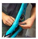
FRAME ASSEMBLY First slide the swing arm over the main pivot as shown. Notice the recess cut in the swing arm in front of the bearings. This recess should be lined up over the main pivot lip to ease the installation process. Place the plastic washers on both sides of the steel pin as shown. While holding the washers in place slide the seatstays over the washers and dogbone.
