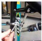
FRAME DISASSEMBLY To remove the shock mounting bolts, place a 5mm allen key on both ends of the bolts and turn counter-clockwise. Once the male bolt is removed, take a 6mm allen key and tap out the female end.
