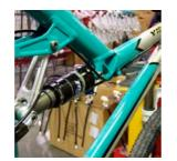
**REAR BRAKE** Run the brake line across the head tube to the first open cable drop out on the non-drive side of the top tube.
