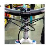
FRONT DERAILLEUR Fit a piece of housing from the front shifter across the head tube into the first cable drop outs on the drive side of the top tube.
