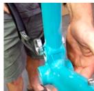
FRAME ASSEMBLY Now slide the 41.2mm female bolt and washer through the seatstays and shock assembly. Place a male bolt with a washer on the opposite side of the female bolt and thread into position. Cinch down both bolts with 5mm allen keys.
