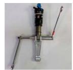
LINKAGE ASSEMBLY While turning the tool make sure you press the shock pin into the correct position. The easiest way to gauge this is to use one of the white nylon washers. The relief on the pin should be even with the washer.
