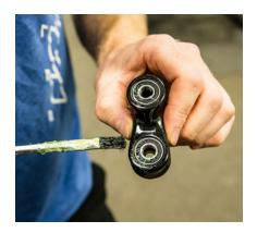
**06.** Lightly grease the bearing surfaces on your link (200020261).
