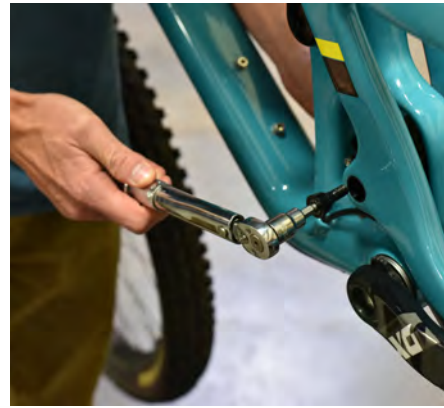
07. Install the Main Pivot Collet Wedge and
