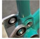
**FRAME ASSEMBLY** Place the black washer over the main pivot pin as shown and thread the male button head on. Cinch the button head down with a 5mm allen key while holding the opposing side with the 6mm allen key.
