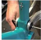
**FRAME ASSEMBLY** Slide the seatstays over the steel pivot pin. Then slide the 41.2mm female Yeti bolt and washer through the seatstays and shock assembly. Place a male Yeti bolt with a washer on the opposing side of the female bolt and thread into position. Cinch down both male Yeti bolts with the 5mm allen keys. The last step is to install the derailleur hanger and water bottle bolts.
