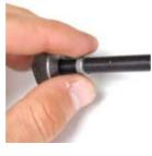
LINKAGE ASSEMBLY Place two of the Dogbone bearings and the 1.38" steel pin onto the threaded bolt as shown followed by a washer and nut.
