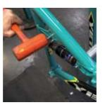
**FRAME ASSEMBLY** Pull the dickey or 8mm allen key out slightly so you can get the 2mm female bolt started. Tap the 22mm female Yeti bolt into position with the dead blow hammer.
