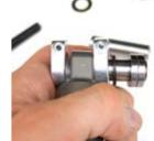
LINKAGE ASSEMBLY Once you have the pin subassembly started into the shock eyelet, you can slide the threaded bolt, press-cup, and press-cup insert configuration from step 1 through the steel pin subassembly and shock. On the opposing end of the bolt slide the second nylon washer, remaining two bearings, press-cup insert, press-cup, washer, and nut.
