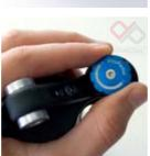
**REBOUND** The rebound adjustment has a 9 click range. As a general rule, adjustments that are too fast (counter-clockwise adjustment) will produce a springy ride with excessive kick up of the rear end. Adjustments that are too slow (clockwise adjustment) will cause packing of the rear wheel and give the bike a sluggish feel.
