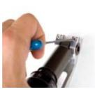
**FRAME DISASSEMBLY** Slide a washer and removal slug onto the threaded bolt. Slide this subassembly through the shock and Dogbone. On the opposing end slide on the catch sleeve, washer and nut. Use 1/2" and adjustable wrenches and torque down until the removal slug presses the steel pin out of the Dogbone bearing assembly.
