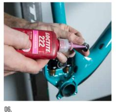
UD. Place the steel washer on the lower link bolt and apply pink Loctite (222).
