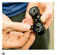
**UD.** Place the bearing race extender washers (300020049) on the lower link bearings. There should be just enough grease there to hold the
