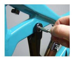
Install the dogbone onto the frame. Insert a 40.5 mm alloy female bolt with washer through the drive side of the frame and the dogbone. The fox guide pin tool and a dead blow hammer can be used help guide any female bolts through the frame and its components. Use an alloy male bolt prepped with purple loctite on the non-drive side and tighten with two 4mm allen keys.
