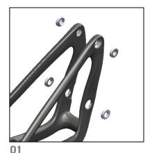
Press 2x 6902-2RS Extended Race bearings (3.17) into the seatstay pivots. Press 2x 6903 bearings (3.16) into the main pivots in the rear triangle.
