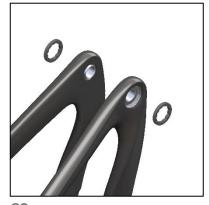
Grease threads of 2x Bearing Lockrings (3.5) and install into the seatstay pivots on the rear triangle. Exercise caution to not cross-
