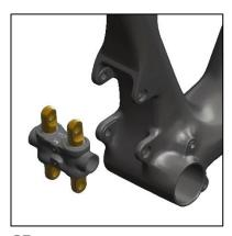
05 Set the Switch Infinity Link (3.2) into the frame. Make sure that the two access screws on the Switch Infinity body are facing outward.
