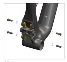
06 Apply Blue Loctite 243 to the threads of 4x M8 Shoulder Bolts (3.6). Begin installing Shoulder Bolts with washers (3.8) through frame and into the Switch Infinity shaft threads. Do not fully tighten - install until 3-4 threads are visible past each Switch Infinity shaft.
