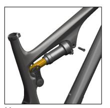
11 Install the rear shock eyelet into the link and secure with a guide pin.
