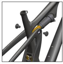
Apply Blue Loctite 243 to the threads of the Seatstay Pivot Bolts (3.22). Install through the Rear Triangle and into the SB115 Link.
