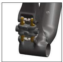
08 Using a wrench to hold the Jam Nuts in place, fully install each M8 Shoulder Bolt until snug.
