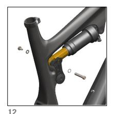
Install 41mm Female Bolt (3.14) with Washer (3.8) through SB115 Link and rear shock eyelet.
