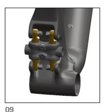
Hold the Shoulder Bolts in place and tighten the Jam Nuts against the Switch Infinity shafts.
