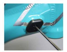
Inset a fork bumper into the recess on the drive side of the frame. Prep a M4x8mm SHC bolt with blue loctite and tighten the bumper to the frame with a 3mm allen key. Repeat the process for the non-drive side.
