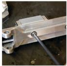
MAIN RAIL SUBASSEMBLY Place the Main Pivot Mount onto the rail as shown. Make sure the threaded mount is positioned away from the grease port. Apply loctite to the two M6x1x8 button caphead bolts and tighten down using a 4mm allen key.
