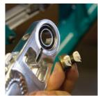
MAIN ASSEMBLY Tap the lubricated pivot pin into the frame with a dead blow hammer. Repeat this process for the second bearing mount on the swingarm.
