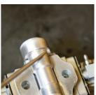
**TOP RAIL SUBASSEMBLY** Apply loctite to the four M5x.8x12 socket caphead mounting bolts.
