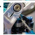
MAIN ASSEMBLY Secure the lower shock mount to the swingarm using the M5x.8x12 and M5x.8x14 socket cap head bolts. The shorter of the two bolts the M5x.8x12 is used for the upper mounting hole and M5x.8x14 is used for the lower mounting holes. Remember to use loctite on the threads and tighten using a 4mm allen key.
