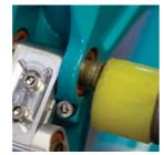
MAIN ASSEMBLY Apply ti prep to the M6x1x12 Ti Male Bolt. Screw the bolt and washer onto the pin as shown and tighten using a 5mm and 6mm allen keys.
