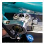
**ECCENTRIC ADJUSTMENT** Once the eccentric mount is in the desired position secure the mounting bolts.
