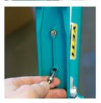
MAIN ASSEMBLY Screw the M5x.8x14 socket cap head bolts into the frame as shown. Don not torque the bolts down, that will take place at a later step.
