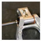
STABILIZING LINK SUBASSEMBLY Place the 38802 2RS Max Bearings into the tail of the Stiff Link H, make sure the extended race is pointing outwards. Slide the 12.7mm x 7mm Pivot Pins into the bearings as shown. Screw the M4x.7x16 socket caphead mounting bolts into the link. Just torque lightly so the bearing and pin assembly does not fall out of the link. The final torque application will take place at a later step.
