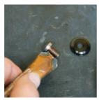
STABILIZING LINK SUBASSEMBLY Attach the Ti Male Bolt and Pivot Pin Washer to the 12mm x 42mm Pivot Pin and tighten using a 5mm and 6mm allen keys.
