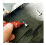
**TOP RAIL SUBASSEMBLY** Place the Eccentric Clamp onto the Eccentric. Apply loctite to the four 6x1x18mm socket caphead mounting bolts, and tighten them into the Eccentric Base using a 5mm allen key.
