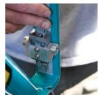
MAIN ASSEMBLY Attach the Main Rail subassembly to the frame with the M5x.8x16 socket caphead bolts. Tighten using a 4mm allen key. Make sure you prep the bolts with loctite.
