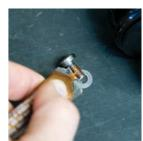
SHOCK LINK SUBASSEMBLY Attach the M6x1x12 Ti Male Bolt and 6.5mmID x 12.5mm0D washer to the female bolt and tighten using two 5mm allen keys. Don not fully torque the complete torque will take place at a later step.
