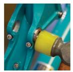
MAIN ASSEMBLY Tap the bearings with the 14mm socket to slightly recess them into the frame.
