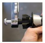
MAIN ASSEMBLY Screw M6x1x12 Ti Male Bolt and Axle Cap onto the axle. Make sure to apply ti prep to the threads.
