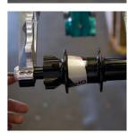
MAIN ASSEMBLY Tighten the pinch bolts on the dropouts using a 5mm allen key. Repeat for the opposing side.
