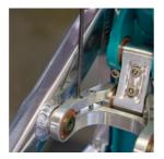
MAIN ASSEMBLY The final steps are to tighten the pinch bolts on the swingarm. Locate the bolts near the bearings and secure using a 5mm allen key.
