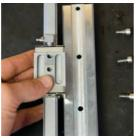
TOP RAIL SUBASSEMBLY Place the Eccentric Base onto the Linear Block. Make sure to place the shorter tab of the Eccentric Base towards the grease port as shown.
