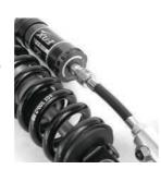
PRO-PEDAL The Pro-Pedal adjustment has a 15 click range of adjustment. The Pro-Pedal damping affects the first half of stroke.
