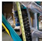
SAG SETUP Next, sit on the bike and record the new (eye-to-eye) measurement. Subtract the static eye-to-eye measurement from this new measurement and you get your sag in inches. An easy way to calculate sag is to multiply the shock travel by your desired sag percentage. See quick setup guide on page 20.
