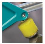
MAIN ASSEMBLY Line up the through holes on the frame and rail mount and slide the 8mm x44mm Solid Ti Female Bolt and 8.5mmID x 2.5mmOD washer through the assembly. Do not attach the opposing male bolt, the female bolt stays in this configuration only temporarily until a later step.
