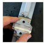
TOP RAIL SUBASSEMBLY Make sure the grease port is at the opposite end the square opening of the Top Rail Mount as shown.
