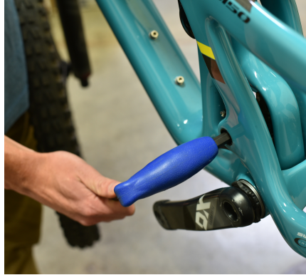
02. With a 10mm allen wrench, remove the Main Pivot Collet Axle. The Collet Nut on the drive side can remain in the frame.
