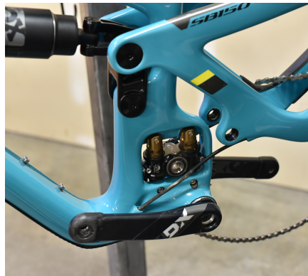
03. Rotate your swingarm upwards to access both grease zerks and expose the whole Switch Infinity link. With a clean rag and mild detergent, clean any mud, dust, or debris off the Switch Infinity Link.
