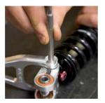
**5 LINKAGE ASSEMBLY** If the Guide Pin does not slide in easily it is appropriate to tap the pin with a dead blow hammer. The pin should slide in with light taps from the dead blow hammer. Do not tap the pin all the way through the assembly as you will need to have the stepped end exposed for next step in the assembly process.
