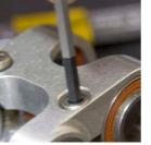
FRAME ASSEMBLY Slide the black Inner Bushing into the IGUS
