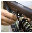
FRAME ASSEMBLY Use two 5mm allen keys to secure the male/ female connection.
