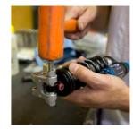
**B** LINKAGE ASSEMBLY Thread the Button Head Bolt (M6 X 1 X 12 mm) on the other end of the Ti-Stud. Once again make sure to apply a small amount of blue Loctite.
