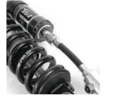
**3 PRO-PEDAL** The pro-pedal adjustment has a 15 click range of adjustment. The pro-pedal damping affects the first half of stroke where most pedal induced bob occurs.
