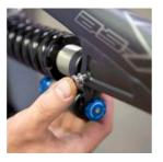
**FRAME ASSEMBLY** Swing the Dogbone up to the preferred travel position and lineup the thru holes on the frame and Dogbone. Slide the Female Yeti Bolt 24.8mm and Washer (8.5 X 12.5 X 0.5 mm) through the frame and shock
