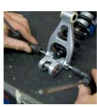
**FRAME ASSEMBLY** One of the Button Heads will break free, remove the Button Head and Washer.
