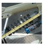
**5** SAG SETUP Next, sit on the bike and record the new (eye-to-eye) measurement. Subtract the static eye-to-eye measurement from this new measurement and you get your sag in inches. An easy way to calculate sag is to multiply the shock travel by your desired sag percentage.
