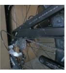
**2 FRONT DERAILLEUR** Fit a piece of housing from the front shifter across the head tube into the first closed cable stop on drive side of the top tube.
