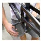
FRAME ASSEMBLY Rotate the swingarm into position over the end 21 of the Shortlink. Slide the Guide Pin through the seatstay mount as shown.
