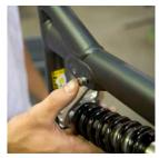
**FRAME ASSEMBLY** Thread the Male Pivot Bolt 17mm and Washer (8.5 X 12.5 X 0.5 mm) into the female bolt. Make sure to apply a small amount of blue Loctite to the threads.
