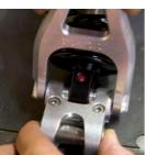
**LINKAGE ASSEMBLY** If necessary use the Yeti Guide Pin to line up the Dogbone, Shortlink and shock eyelets by sliding the Guide Pin through the sub assembly.
