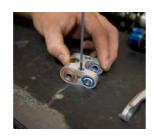
**LINKAGE ASSEMBLY** Slide the u-shaped end of the Shortlink over the back end of the shock. Make sure you slide the Shortlink over the proper end of the shock with the rebound knob facing down and the pinch bolts facing up.
