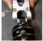
**3** LINKAGE ASSEMBLY Slide the Dogbone over the outside of the Shortlink. Line up the thru hole of the Dogbone with the inner race of the bearings.
