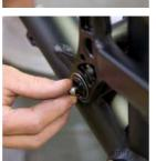
**FRAME ASSEMBLY** Place a 5mm allen key on the Button Head bolt and a 6mm allen key into the main pivot pin and secure.
