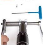
FRAME DISASSEMBLY To remove the main pivot pin, place a 5mm allen key on the button head bolt and a 6mm allen key on the pivot pin. Turn counter-clockwise until the button head is removed. Then take an 8mm allen key and tap out the main pivot pin.
