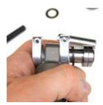
LINKAGE ASSEMBLY Once you have the pin subassembly started into the shock eyelet, you can slide the threaded bolt, press-cup, and press-cup insert configuration from step 1 through the steel pin subassembly and shock. On the opposing end of the bolt slide the second nylon washer, remaining two bearings, press-cup insert, press-cup, washer, and nut.
