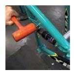
FRAME ASSEMBLY Pull the dickey or 8mm allen key out slightly so you can get the 2mm female bolt started. Tap the 22mm female Yeti bolt into position with the dead blow hammer.
