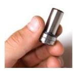
LINKAGE ASSEMBLY Place the Dogbone over the shock with the counter-bored holes facing the lever of the shock, and the threaded end of the hold facing away from the shock. Slide the pin sub assembly into the shock eyelet as shown.
