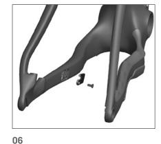
Install the Chainstay Cable Port Cover (2.7) to the non-drive side chainstay port and secure with Flat Head M4 x 10L. Hardware can be torqued to 2-3 Nm after housing installation.
