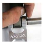
FRAME ASSEMBLY Place the shock assembly onto the bike in the configuration shown to the right. Slide the 5/16 dickey or 8mm allen key through mounting position one to hold the shock assembly in place. Swing the Dogbone into mounting position two. Slide a 22mm female Yeti bolt and washer through the mounting hole. Tap the 22mm female Yeti bolt into position with the dead blow hammer.
