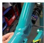
FRAME ASSEMBLY Slide the rear triangle over the main pivot as shown. Notice the recess cut in the swingarm in front of the bearing. This recess should be lined up over the main pivot lip to ease the installation process. Make sure the bearings are lined up with the main pivot bore before tapping the lightly greased main pivot pin through the frame with the dead blow hammer.
