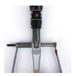
LINKAGE DISASSEMBLY Place the wrenches on the tool assembly and turn to press the pin out.
