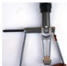
FRAME DISASSEMBLY To remove the main pivot pin, place a 5mm allen key on the button head bolt and a 6mm allen key on the pivot pin. Turn counter-clockwise until the button head is removed. Then take an 8mm allen key and tap out the main pivot pin.
