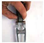
LINKAGE ASSEMBLY Slide a washer on the threaded bolt then slide this through the removal slug (1.5" long). Then slide on the shock pin. Slide the tool assembly through the Dogbone, shock connection point. On the opposing side slide on the catch sleeve and washer, then thread the nut on. Place the wrenches on the tool assembly and turn to re-set the shock pin.
