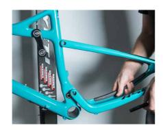
**08.** Slide the swing arm into place over the main pivot sleeve on the front triangle.
