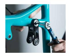
**06.** Finish tightening the upper link pivot using a well calibrated torque wrench set to 5 Nm
